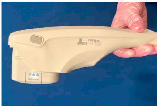
Fig. 1. Ulthera handpiece with interchangeable transducer (4 MHz, 4.5 mm treatment depth transducer shown). (Photo courtesy of Merz Aesthetics/Ulthera.)
